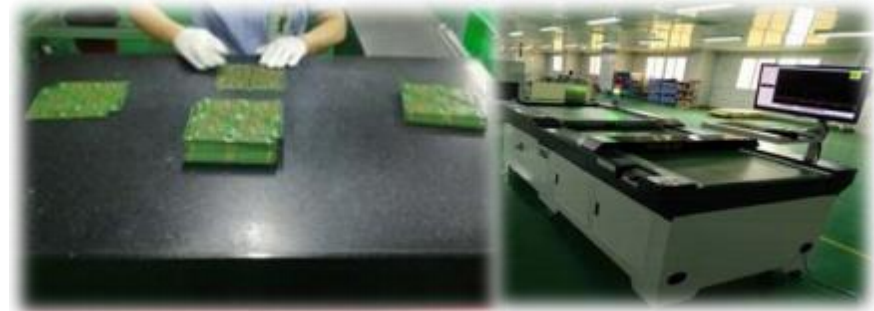
Two confirmation of warping, automatic board warping inspection before shipment
